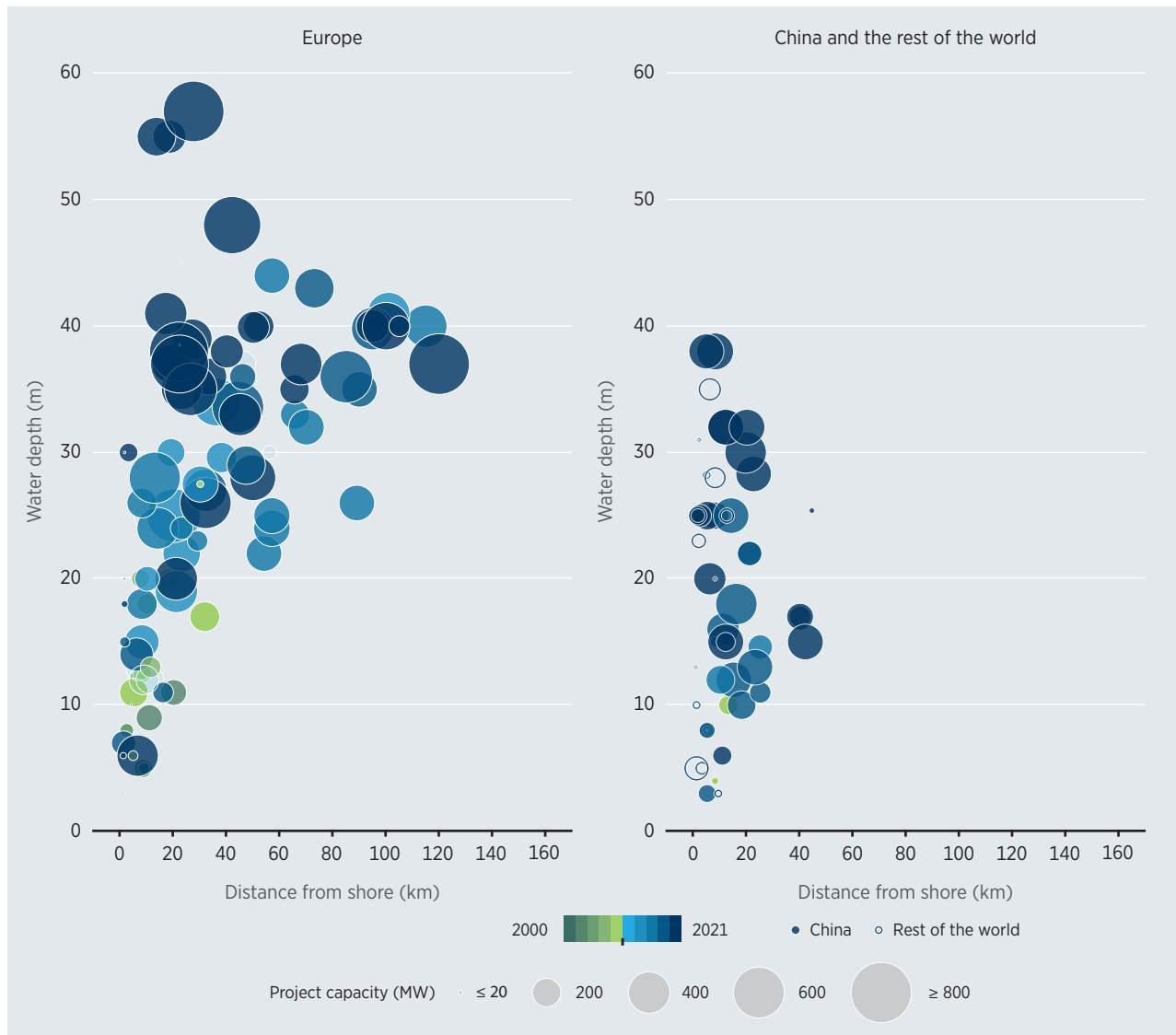
Figure 4.2 Average distance from shore and water depth for offshore wind in China, Europe and the rest of the world, 2000-2021
